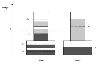
In this figure, each job is described by a rectangular container. The height of the container is the weight of the job, and its area is  $2^{j+1}$  for bin  $A_j$ . The area of the gray rectangles inside each container represent the volume of the job. The container is separated into two halves by a dotted line.
